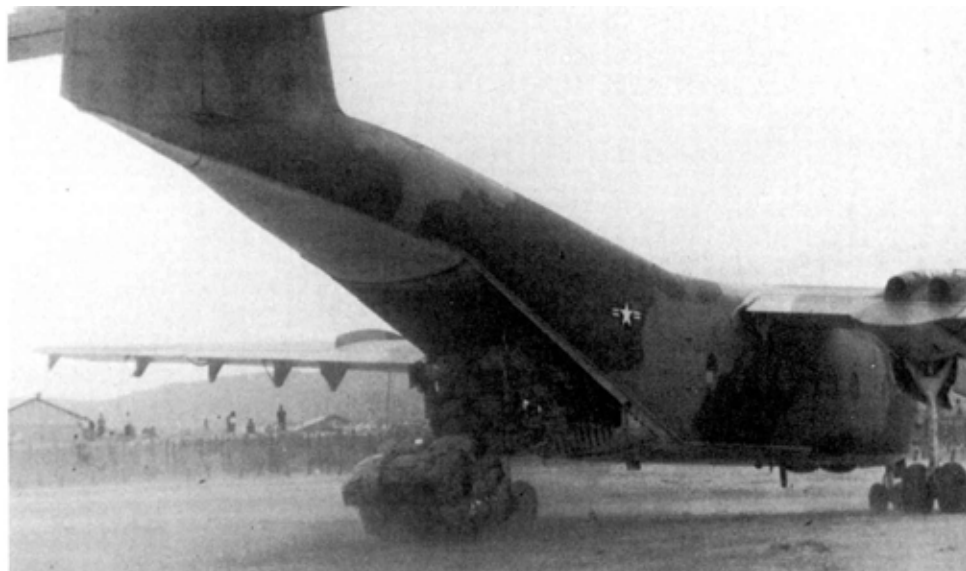
There are many techniques for getting cargo out of the Caribou . At Dak Seang, a remote Special Forces camp, the crew demonstrated the Ground High Speed Offload method. As the Caribou lurches forward, pallets fly out the rear door. Pallets held fiber bags for sandbagging the fort .
