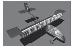
The FanWing experimental aircraft opens up a new area of aerodynamics. Designs to establish a means of integral lift and thrust using a horizontal-axis wing rotor are recorded back as far as the late 19<sup>th</sup> century. Some of the experiments started to take off but did not sustain flight. The FanWing new blown-wing solution offers both basic proof of concept and improved and controlled flight performance.
