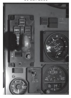
The photo above shows the gear handle of the C-17 which landed gear-up at Bagram, Afghanistan. The crew was making a combat approach into the airfield and there were 3 pilots on board the aircraft. They were taking ground fire at the time of the incident and became distracted with all the commotion of what was going on outside the airplane. They took many hits from small arms. The Aircraft Commander had a total A/C time of 200 hrs and the other two pilots were about the same.
