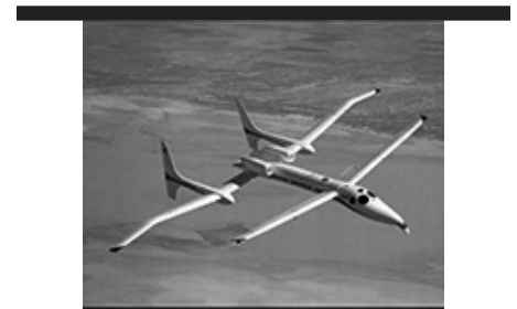
Proteus , a tandem wing, twin-engine research aircraft built by Scaled Composites, 1998
