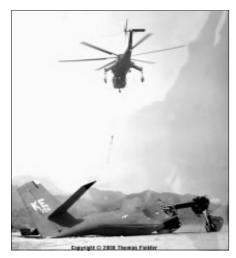
After hitting the ground, the Caribou broke in half forward of the troop doors. As the main gear then hit the ground the engines broke their mounts and also tumbled to the ground.
