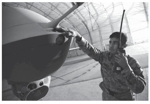
Data Link and Tactical Common Data Link antennas, plus radio frequency equipment.
