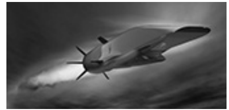
The hypersonic X-51 Waverider vehicle has reached Mach 5.1 speed in a six-minute flight.
